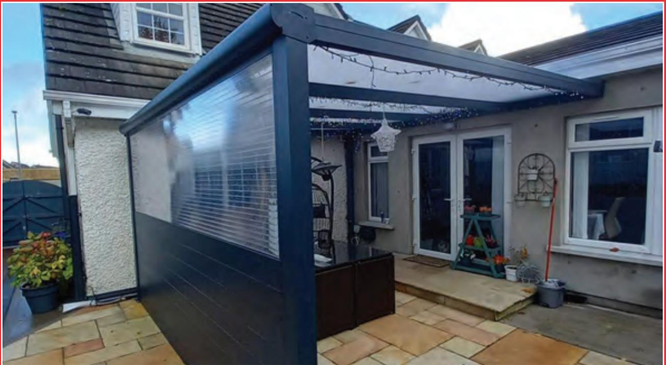
Here is an example of a 4m x 4m Bosco veranda installed in a corner with one side closed off to create additional shelter. This wall is aluminum
